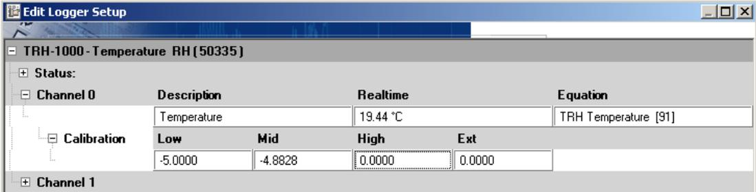
The screenshot shows the 'Edit Logger Setup' window for a TRH-1000 Temperature RH (50335) logger. The window is divided into sections for Channel 0 and Channel 1. Channel 0 is expanded to show its calibration settings. The 'Description' is 'Temperature' and the 'Realtime' value is '19.44 °C'. The 'Equation' is 'TRH Temperature [91]'. The 'Calibration' section is expanded to show four fields: 'Low' (-5.0000), 'Mid' (-4.8828), 'High' (0.0000), and 'Ext' (0.0000). Channel 1 is collapsed.
