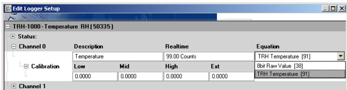
Some channels compensate their output by using the value of another channel. For example, the calculated value for an RH channel depends on the reading of the RH sensor and the value of the temperature channel. In such cases, the compensation channel must output in the correct units. In the case of RH, for example, the temperature channel must output in units of temperature. Using units of byte counts will give invalid results.
